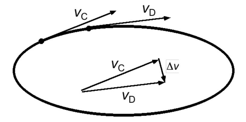
As point D is moved closer to C, angle approaches 90°.
