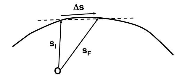
$v = \Delta s / \Delta t$  lies along dotted line. As  $\Delta t \rightarrow 0$ direction of v is tangent to path
