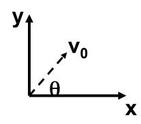
$v_{0y} = v_0 \sin(\theta)$  $v_{0x} = v_0 \cos(\theta)$
