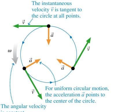
Acceleration vectors for ball swung in a horizontal circle at *constant* speed v
