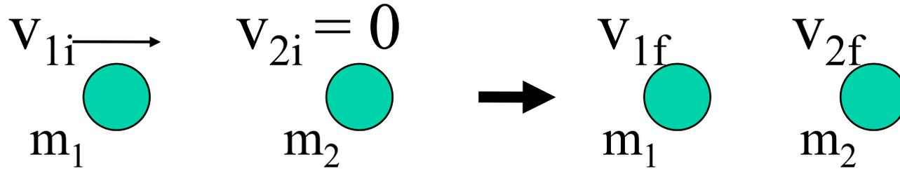
$$\textit{Momentum} \rightarrow m_1 v_{1i} + 0 = m_1 v_{1f} + m_2 v_{2f}$$
