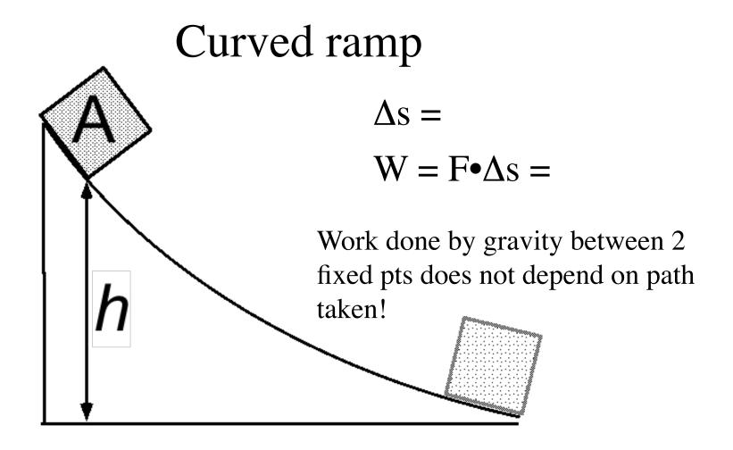
Work done by gravitational force in moving some object along any path is independent of the path depending only on the change in vertical height
