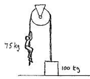
a. [5 pts] Draw the free-body diagrams for the person and for the block, labeling all of the forces acting on each. Make sure to label which free-body diagram is which.
